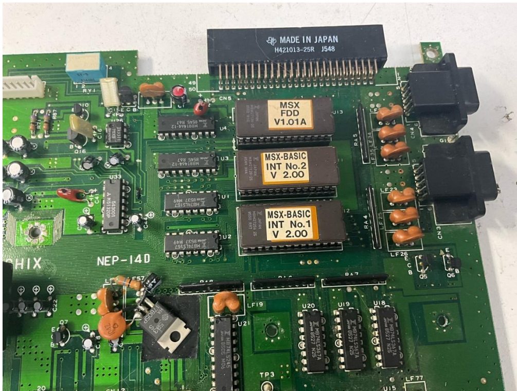
The original disk ROM, U13, in the IC socket.
