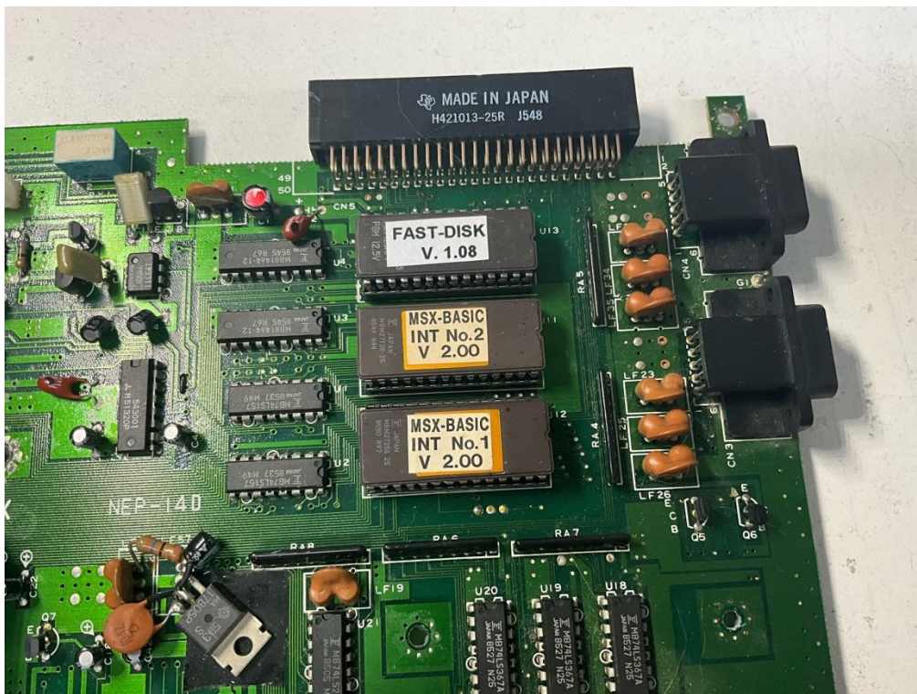
The new disk ROM is placed in the IC socket of U13.
